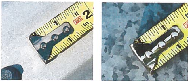
Differing spangles of galvanized (left) and Galvalume (right). (Author's photos)
