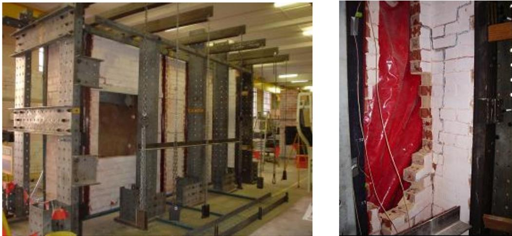
(a) overall view of test set-up (b) failure by collapse of brick units
