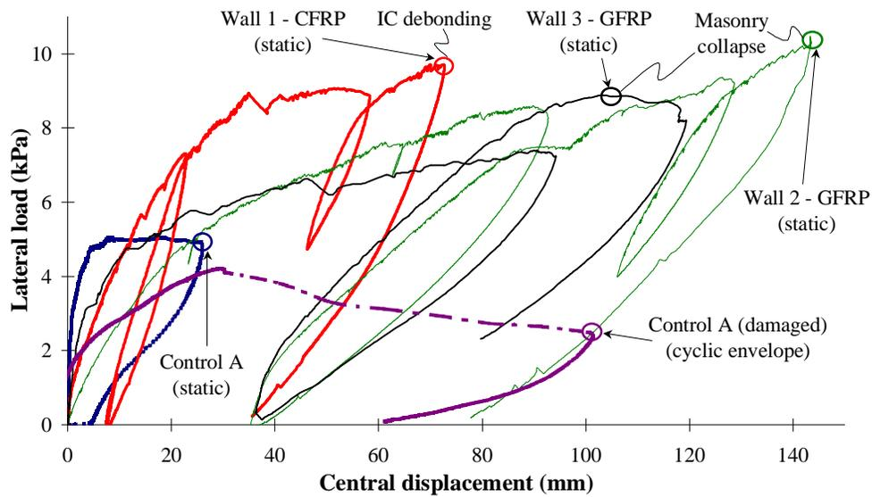
Figure 6. Out-of-plane load-displacement response of FRP strengthened URM walls
