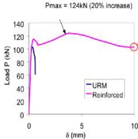
Figure 9. Comparison of typical load-displacement response
