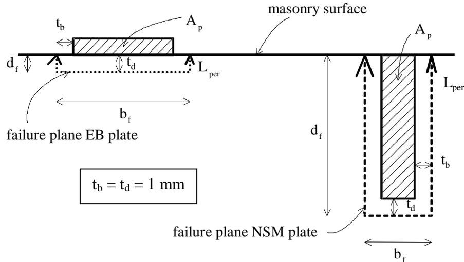
Figure 4. Definition of IC debonding failure plane (cross-section shown)
