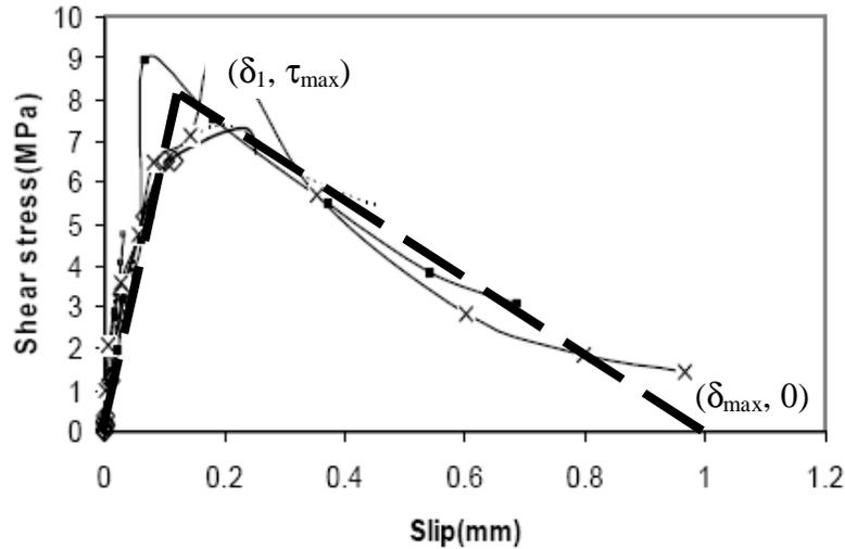
Figure 3. Typical bond-slip relationship of adhesively bonded FRP-to-masonry joints
