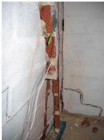
Figure 7. Premature debonding failure of NSM Carbon FRP strip
